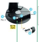
Ref. 40.054.327 patch cable, 3 m with RJ45 connector (8/8-pin), central unit <--> microphone loudspeaker unit Ref. 40.054.376 patch cable, 3 m with RJ10 connector (4/4-pin), microphone loudspeaker unit <--> GN9330e base station
